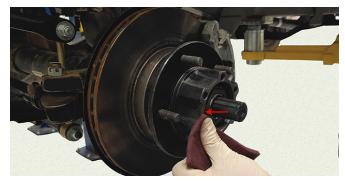
6. Lightly lube warn locking hub seal and install.
