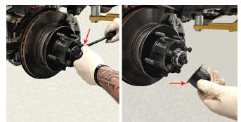
3. Remove snap ring from outer hub at axle end. Remove (6) bolts. Retain snap ring and retain bolts.
