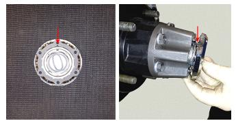
9. Finger Tighten (5) Allen Bolts, then torque to specification.
