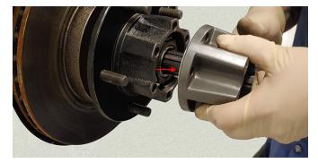
7. Reusing original fasteners, torque to specification. Reinstall Snap Ring (apply outward pressure to axle if necessary).
