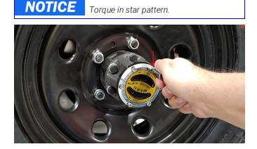
10. Install Wheel and Finger Tighten (5) Lug Nuts, then torque to specifications. Repeat steps for opposite side.
