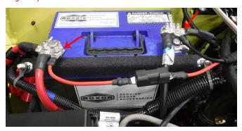
16. Zip-tie all wire harnesses on interior and exterior as necessary (about every foot is recommended) to secure in place.
