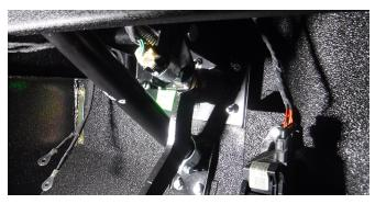
7. Install ROXPOWER to mounting bracket with (4) M6 torx flange screws in locations shown.
