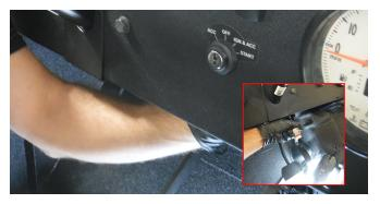
7. Using screw-driver, remove orange wedge from connector. Pull middle red plug (number 5 ) from connector, use pliers if needed.
