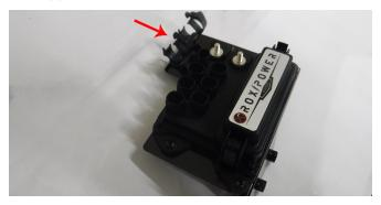
10. Remove side plugs from drivers side of vehicle and discard.
