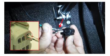
12. Insert 2 pin connector into open ROXPOWER 2 pin socket labeled INPUT.
