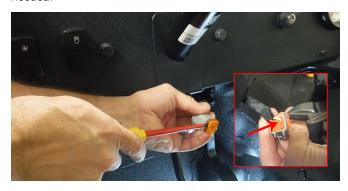
8. Insert white wire into cavity 5 where red plug was removed, push until it clicks. Pull to verify, reinstall orange wedge, plug ignition switch back in.
