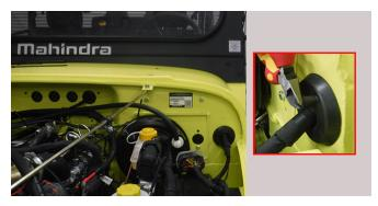
5. Carefully route retro-fit wire harness through nipple hole. Secure to main harness with zip-tie to prevent contact with body. Trim off excess zip-tie.
