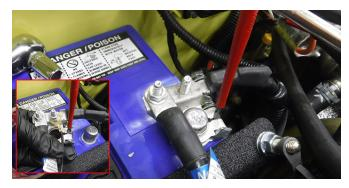
3. Secure clamp terminal so as not to allow it to contact battery.
