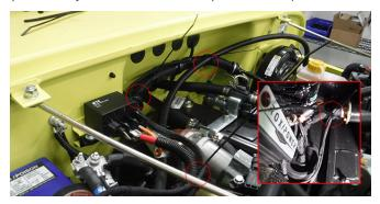
17. Secure negative battery clamp terminal, torque to specifications. Make sure battery clamp is fully seated down to battery before torquing terminal.
