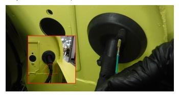
6. Remove ignition switch connector from behind instrument panel.
