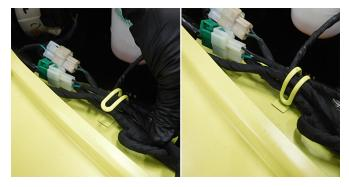
3. Route and wrap the retro-fit wire harness around existing wire harness toward cab.
