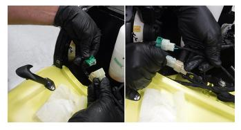
2. Secure harnesses down using existing tab.
