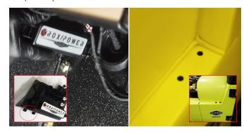
Secure wires into omega-clips at the top of ROXPOWER bracket to prevent wires from falling into pedal area.
