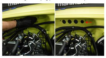
5. Route power harness (end without fuse) through grommet plug hole and seat grommet.
