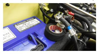
4. Remove first grommet plug (closest to driver side).
