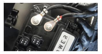
12. Locate 2 pin connector taped to accessory switch wires left of steering wheel. Plug into 2 pin socket labeled INPUT on ROXPOWER. Plug in all accessory features at this point.
