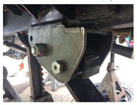
Use the 2 inch hole saw to drill a hole to insert the new rear spring bushings
