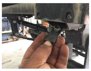
• Loosely bolt the bottom plate into place. Then add the front frame plate so they line up. Once everything is lined up and bolted tightly into place, weld the 2 pieces together. The fitment may take some grinding and fitting. Not all Roxors are aligned the same from the factory.
