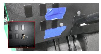
Attach (2) Mounting brackets to ROPS Clamps with (2) M6 Screws torque to specification.
