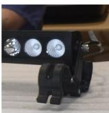
5. Secure Light Bar to A pillar ROPS, with (2) ROPS Clamps and connect ROPS Harness to Light Bar Harness.
