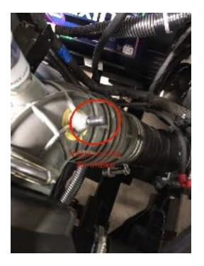
**Step 9:** Using the 10mm socket, remove the vacuum solenoid and bracket along with the vacuum canister and hoses. Zip tie both electrical connecters that were unplugged in step 2 back out of the way as they are no longer used.
