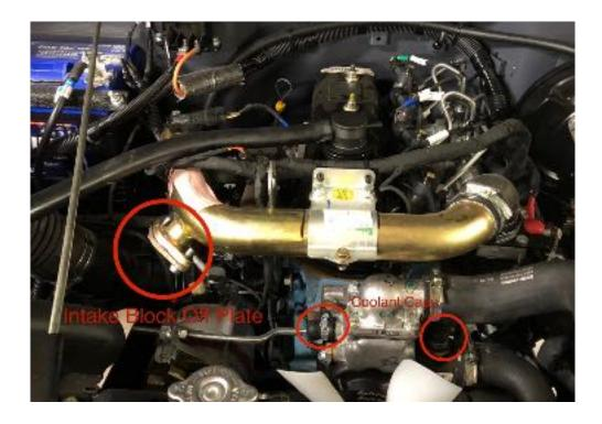
**Step 7:** Install the supplied 5/8" coolant caps on the nipple on both sides of the water pump and secure using supplied hose clamps, not the original spring clamps. Refill coolant.
