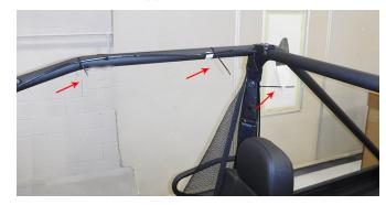
Use (2) zip ties to secure ROPS Harness to B pillar top and bottom. Trim excess from zip ties.
