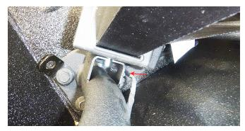
7. Route ROPS Harness up inside B pillar, under existing hook and loop fasteners.
