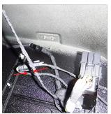
Route ROPS Harness along passenger side of vehicle, attaching (5) Medal Panel Clips to edge.
