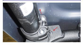
9. Route ROPS Harness along inside top side ROP to front A pillar and secure with (2) Zip Ties.
