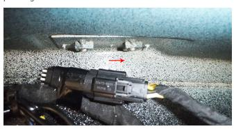
2. Plug connector for ROPS Harness into this plug under passenger side Dash Panel.
