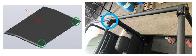
**Step (4)** Install the Rear Roof on the unit by lining up the rear holes in the Rear roof with the rear factory bolt locations of the roll bar, as shown below. Then install the factory bolts with the (4) 3/8" Seal Washers. Make sure these bolts are threaded but not tightened.
