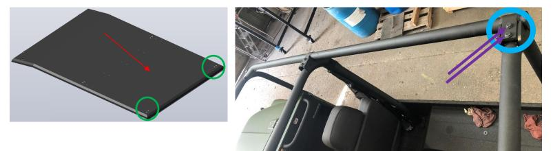
**Step (5)** Remove the front factory bolts and install (2) Front Brackets with the following hardware at the highlighted locations below: <u>Leave loose</u> if you are also installing our <u>vented windshield</u>.
