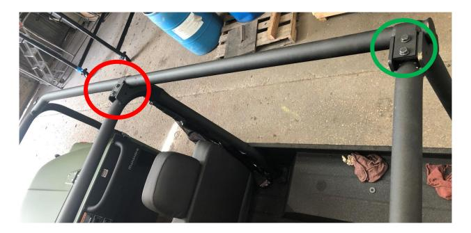
**Step (2)** Install the 45" piece of foam tape and the (2) 65-1/2" pieces of foam tape on top of the roll bar at the highlighted locations pictured below.
