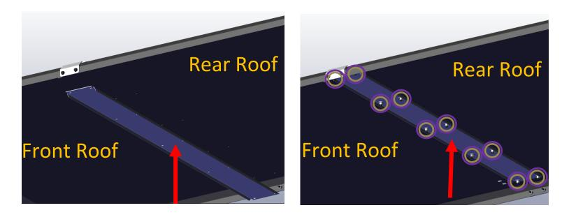
**Step (8)** Finish installing the Upper Seal Plate on the unit by lining up the 2 side holes in the Upper Seal Plate with the 2 holes in the Front and Rear Roof locations as shown below. Then install the (4) 1/4" Nylon Locknuts with (4) 1/4" x 1/2" Bolts as shown below.
