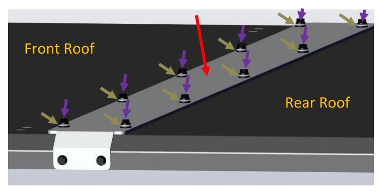
**Step (7)** Install the Lower Seal Plate on the unit by lining up the 10 center holes in the Lower Seal Plate with the 5 holes in the Front and Rear Roof locations as shown below. Then install the (10) 1/4" Nylon Locknuts with (10) 1/4" Flat Washers on to the previously installed 1/4" x 1" bolts.
