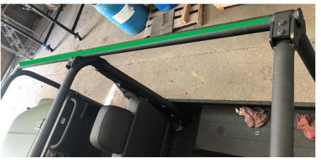
**Step (3)** Install the Front Roof on the unit by lining up the rear holes in the Front roof with the middle factory bolt locations of the roll bar, as shown below. Then install the factory bolts with the (4) 3/8" Seal Washers. Make sure these bolts are threaded but not tightened.
