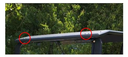
**Step (1)** Remove the (4) rear factory bolts and (4) front factory bolts, from the roll bar, from the highlighted location as shown below.
