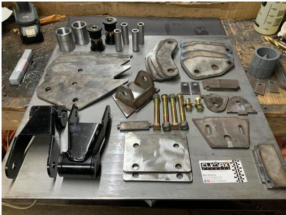
**\*Remove stock suspension, front drive shaft, and front bumper. Save 6 of the shackle bolts.**
