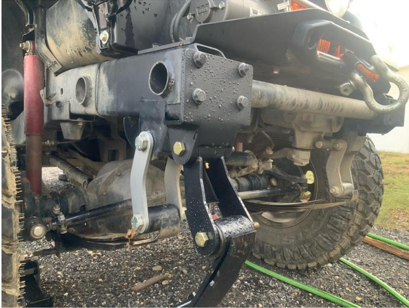
Moving back to the spring hangers at the rear of the front springs...
