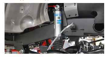
Collapse shock until aligned with lower shock mount, then carefully slide shock onto lower bolt. Install (1) washer and (1) nut removed earlier.
