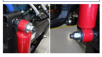
2. Install new shock by loosely securing upper shock mount first with (1) washer and (1) nut removed earlier.
