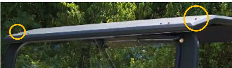
**Step (6)** Install the **Upper Seal Plate** on the unit by lining up the **10 center holes** in the **Upper Seal Plate** with the **5 holes in the Front and Rear Roof locations** as shown below. Then install the **(10) 1/4" x 1" bolts** with **(10) 1/4" Seal Washers** through the **Upper Seal Plate** and then through the **Front and Rear Roofs**.
