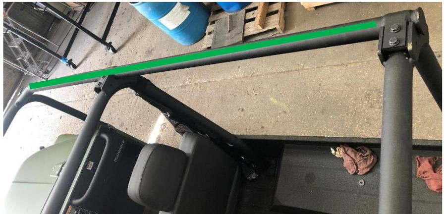
**Step (3)** Install the **Front Roof** on the unit by lining up the **rear holes** in the **Front roof** with the **middle factory bolt locations** of the roll bar, as shown below. Then install the **factory bolts** with the (4) **3/8" Seal Washers**. Make sure these bolts are threaded but not tightened.
