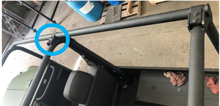
**Step (4)** Install the **Rear Roof** on the unit by lining up the **rear holes** in the **Rear roof** with the **rear factory bolt locations** of the roll bar, as shown below. Then install the **factory bolts** with the (4) **3/8" Seal Washers**. Make sure these bolts are threaded but not tightened.
