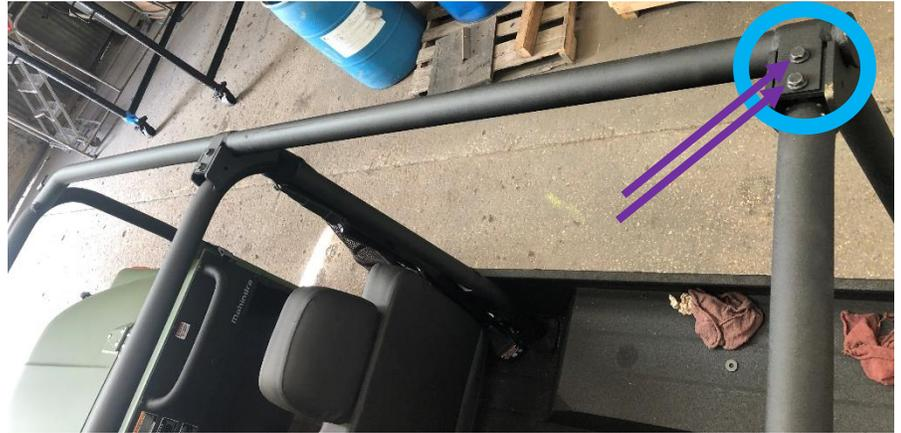
**Step (5)** Remove the **front factory bolts** and install (2) **Front Brackets** with the **following hardware** at the **highlighted locations** below: **Leave loose if you are also installing our vented windshield.**
